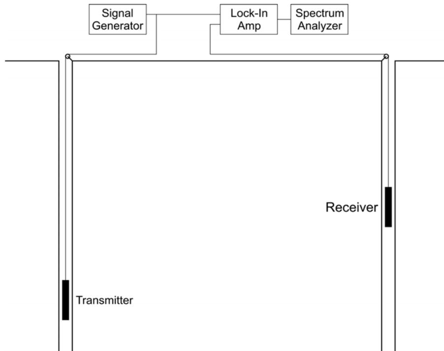
Figure 1: Schematic diagram of a crosshole EMT data acquisition system.
