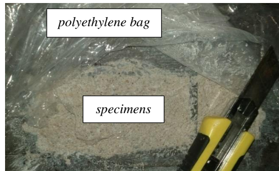
Figure 6-5 – Opening process in the cubic specimens (polyethylene bag)
