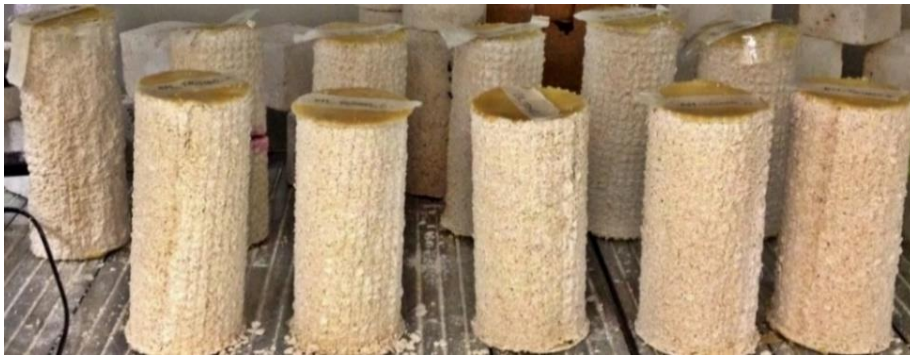
Figure 6-7 – Storage of cylinders (TGA + elastic modulus specimens in part B )
