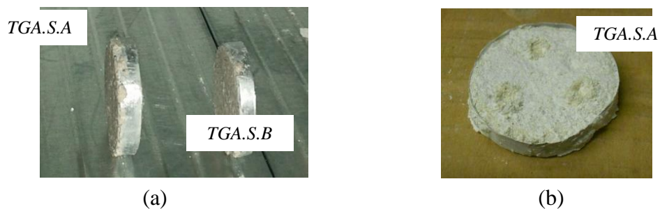
Figure 6-21 – Discs specimens for TGA (a) storage, (b) after sampling
