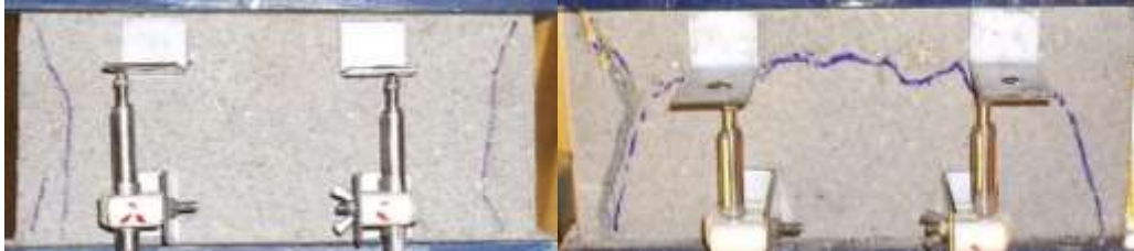
Figure 4 – Crack patterns of concrete blocks under uniaxial compression
