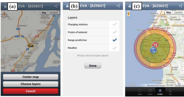
Fig. 9. Range prediction process: (a) FEV position; (b) Available functions; (c) Range prediction representation: green, orange and red.
