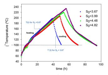
**Fig. 2.** Heating and cooling temperature profiles of autohydrolysis assay carried out at  $S_0 = 3.67, 3.99, 4.48$  and 4.82. Temperature was controlled with a thermocouple inserted in a thermowell, which extends near the bottom of the reactor vessel (T (t): heating profile, T<sup>'</sup> (t): cooling profile,  $T_{REF}$ : temperature of reference, 100 °C).
