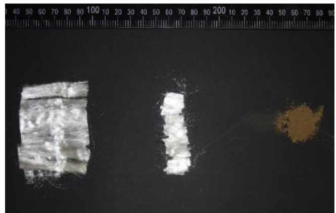
Fig. 9. Visual comparison between the same weight of both types of fibres and soil.
