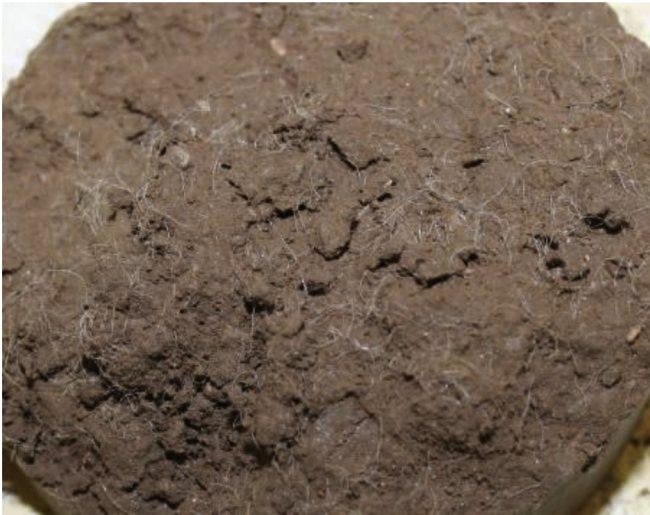
Fig. 6. General view of the fibres' distribution after moulding one of the D.1.1 specimens.
