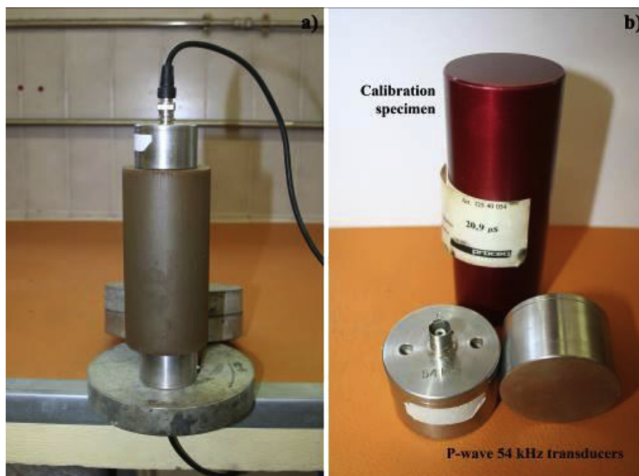
Fig. 7. Setup for the wave velocity measurement (a) and detail of the transducers and calibration specimen (b).
