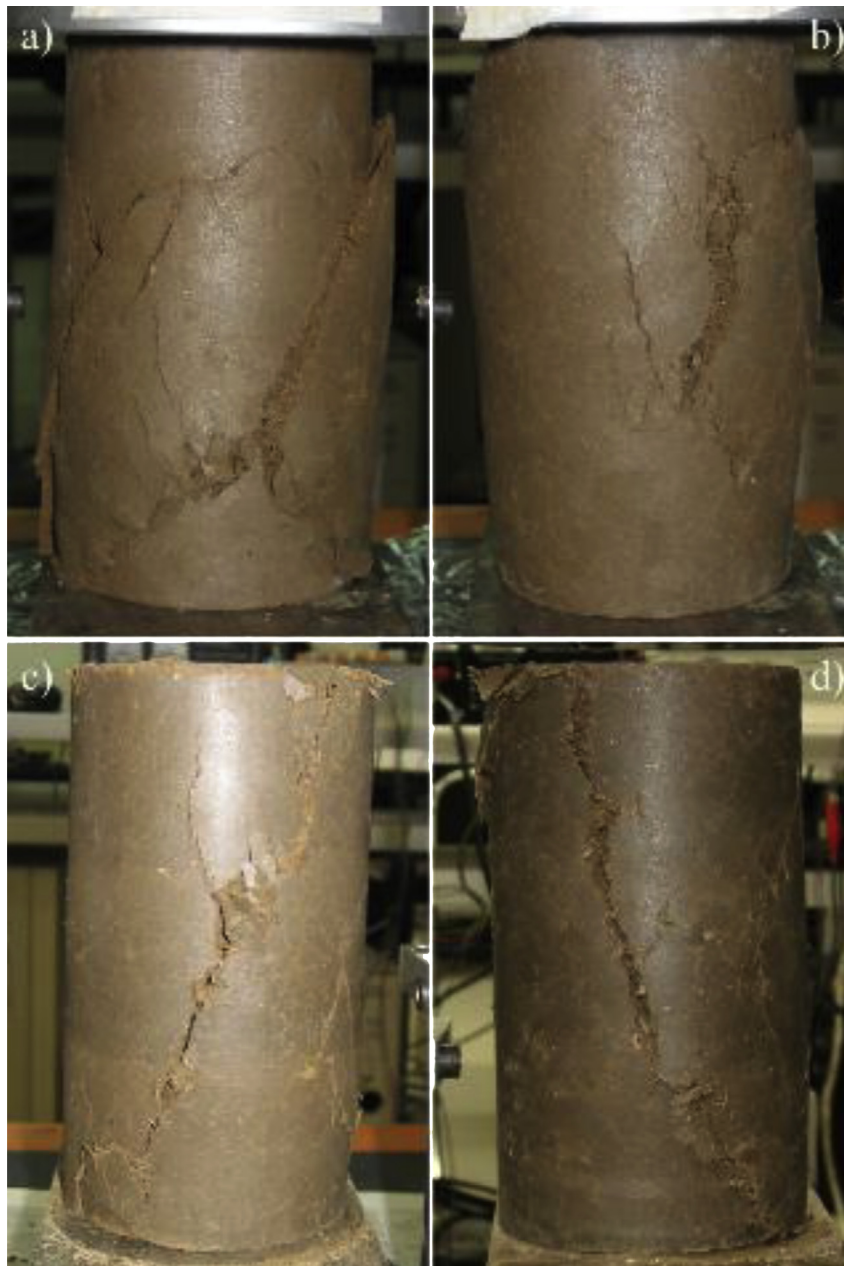
Fig. 21. Effect of fibre content (0.10% and 0.25%) at 75% of the peak stress on 0% cement specimens (a), (b); and 10% cement specimens (c), (d).
