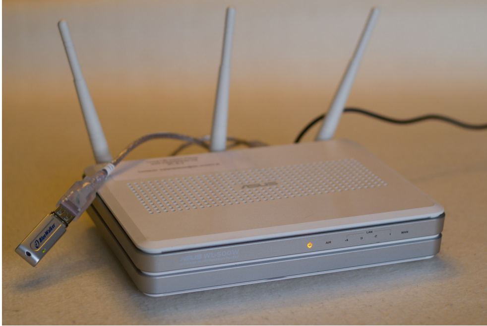
Figure 5.1. An Ethernet router (equipped with an USB Bluetooth dongle) running a prototype of the Bluetooth Hotspot software on OpenWrt Linux.
