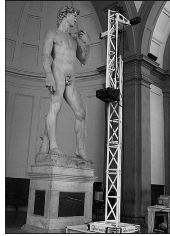
Fig. 160: Laser scanner 3d (Levoy, 1999)
