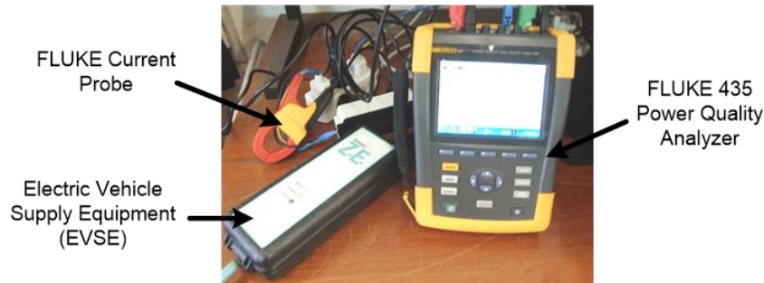
Fig. 2. Setup used for monitoring the battery charging process.
