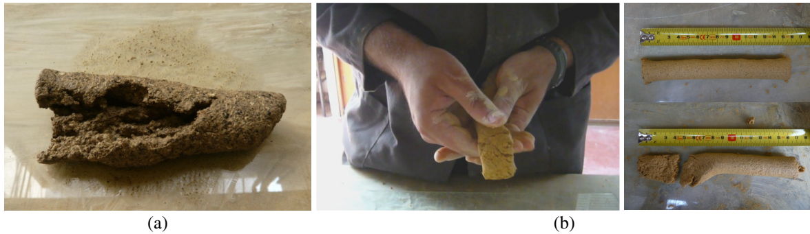
Fig. 3 – Ribbon test: (a) soil S1; (b) soil S4.
