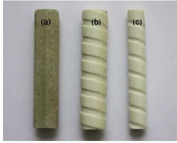
Figure 2 - GFRP bars: (a) Sand-coated 12 mm diameter (type B), (b) Ribbed 12 mm diameter (type A), (c) Ribbed 8 mm diameter (type A)
