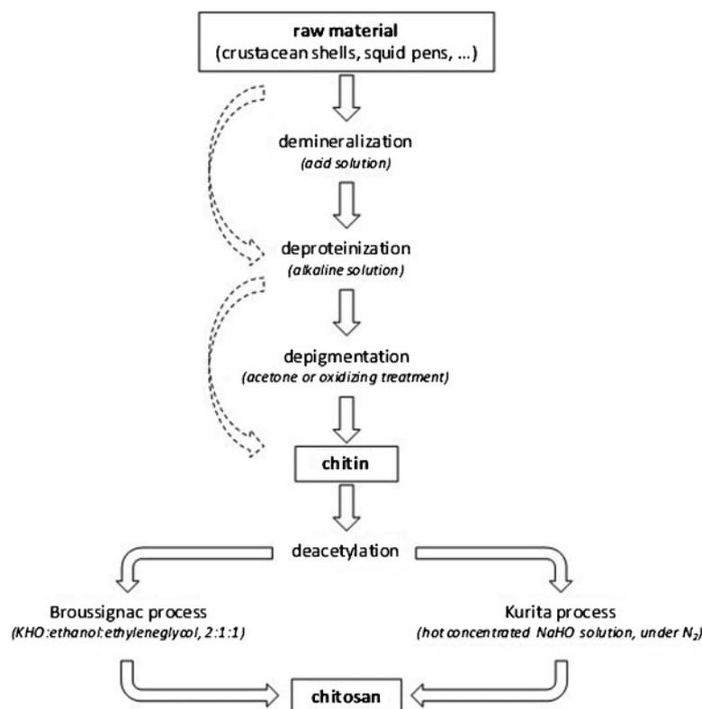
9 Scheme of common process for isolation of chitin from raw materials such as crustacean shells and squid pens (dashed arrows) and its further conversion into chitosan
