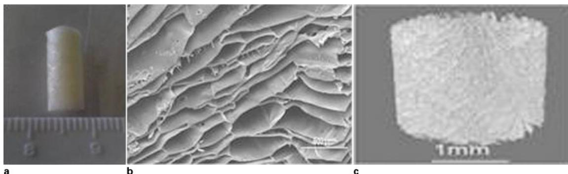
26 Photo of freeze-dried and neutralised chitosan scaffold (a) and respective SEM image (b) and microcomputed tomography image (c)
