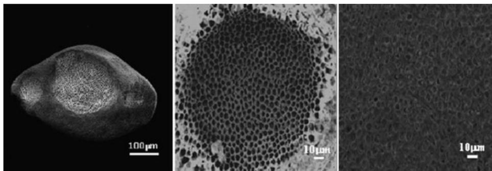
18 SEM images of *Corallina*-derived hydroxyapatite after conversion process developed by Walsh *et al.* (reprinted from Ref. 223 with permission from Elsevier)
