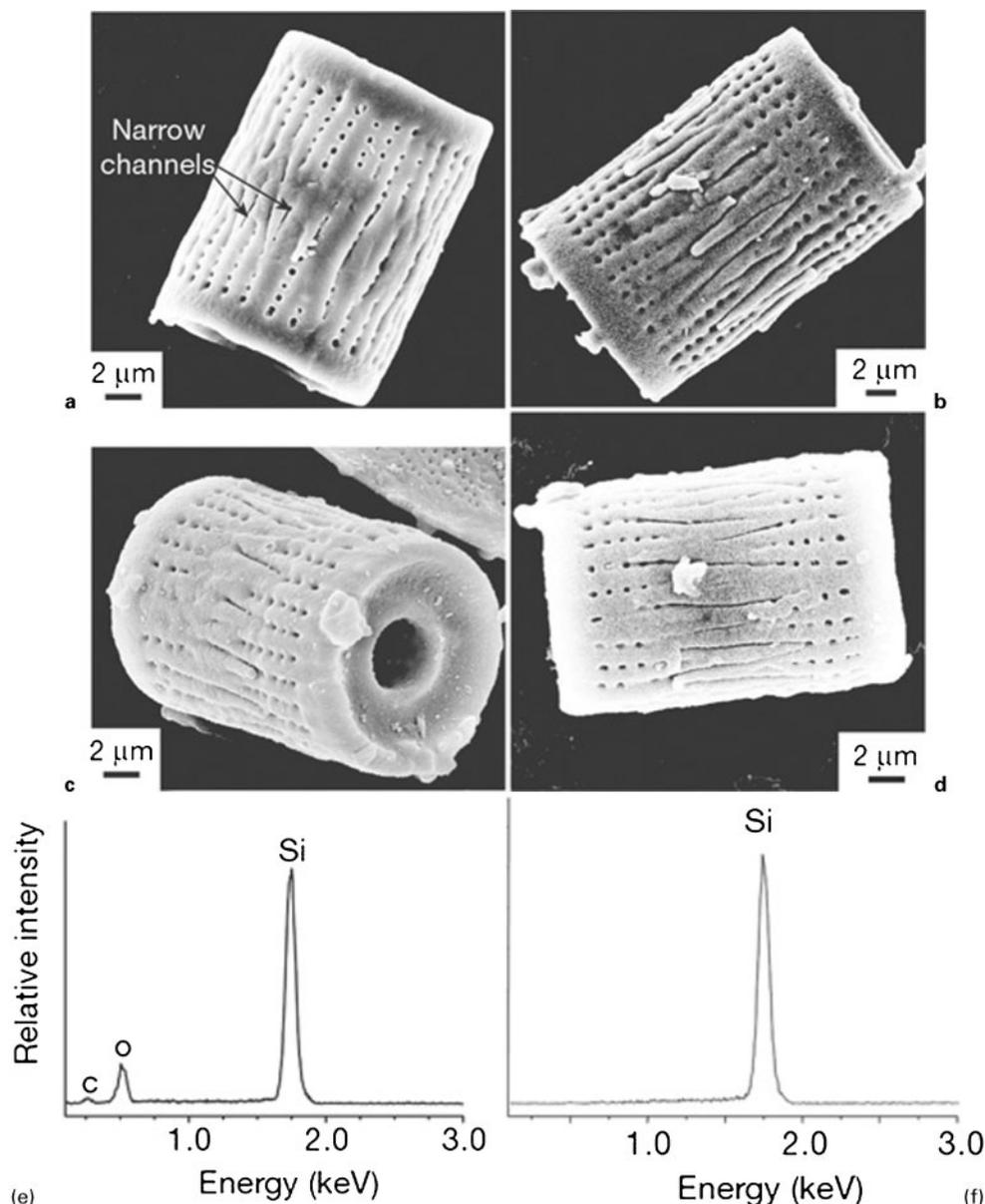
22 SEM images of *a* *Aulacoseira* diatom frustules, *b* MgO/Si replica obtained after reaction of frustule with Mg at 650°C, *c* silicon-based replica produced after treatment with HCl solution and *d* silicon replica obtained after additional treatment with HF solution. *e* and *f* are the results of the energy dispersive X-ray analysis of silicon-based replicas shown in *c* and *d* respectively (reprinted from Ref. 263 with permission from Nature Publishing Group)
