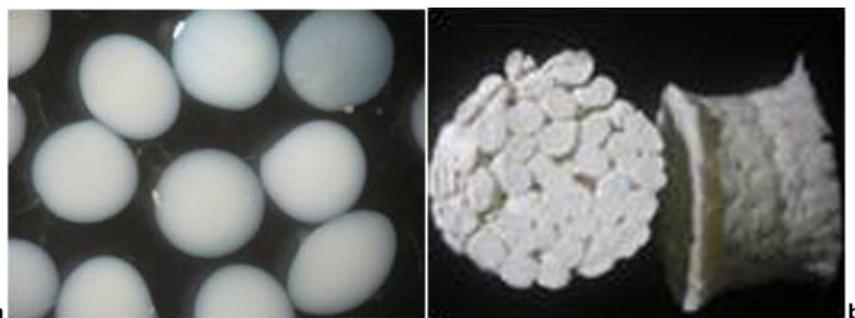
27 Photos of (a) chitosan particles prepared by precipitation of droplets of chitosan solution into an alkaline coagulation bath, which can be agglomerated forming a porous structure (b)
