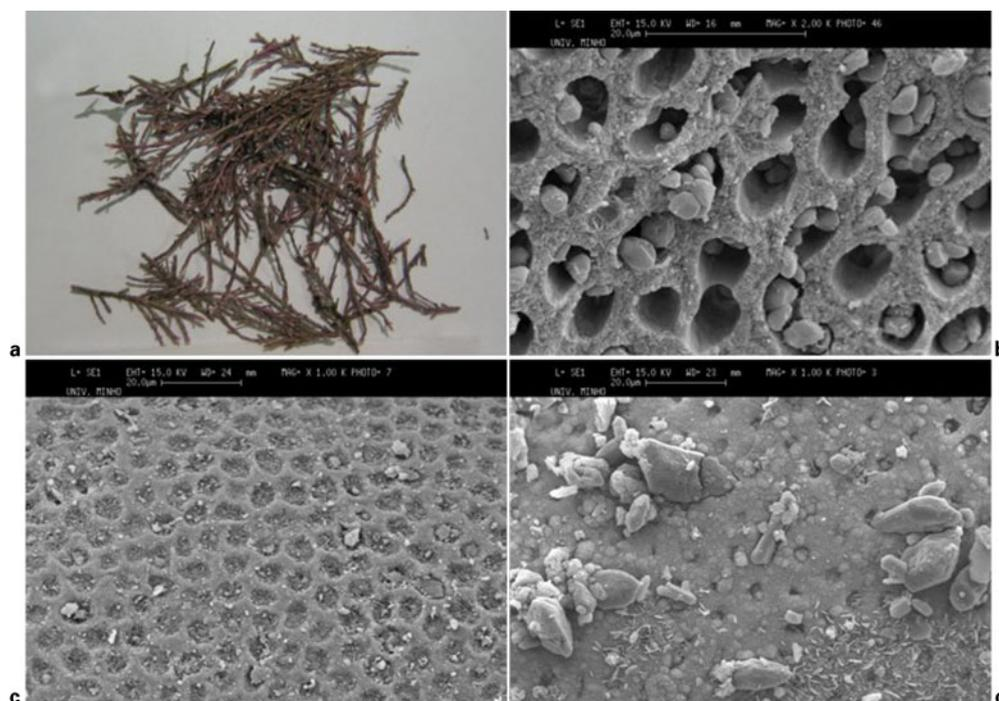
17 Photos of *Coralline officinalis* red algae used as source of calcium carbonate: *Coralline officinalis* (a), SEM image of *Coralline officinalis* (b), SEM image of *Corallina* after heat treatment at 400°C for 3 h (c) and SEM image after heat treatment at 400°C for 3 h, followed by chemical treatment with ammonium phosphate dibasic (d)
