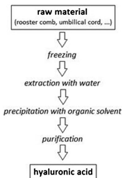
15 Scheme of extraction of hyaluronic acid from raw materials such as rooster combs and umbilical cords, according to the procedure described by Balazs<sup>176</sup>
