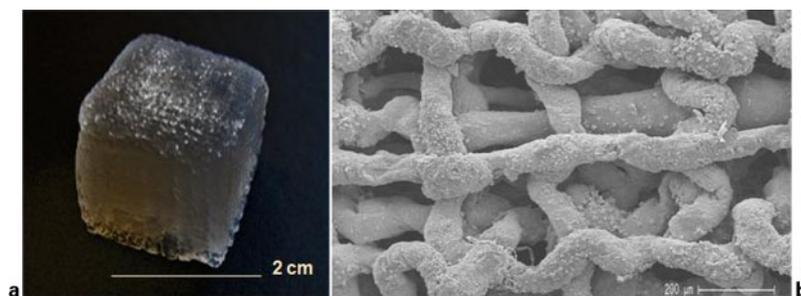
28 Photo of carrageenan scaffold produced by rapid prototyping (a) and respective SEM image (b)
