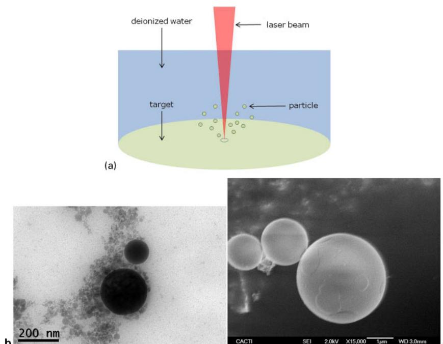
19 a cartoon of the laser ablation process in deionised water for production of calcium phosphate particles, b HRTEM image and c SEM image of calcium phosphate submicro- and microparticles respectively, obtained from fish bones by using laser ablation technique (micrographs reprinted from Ref. 226, Open Access article distributed under the terms of the Creative Commons Attribution License)
