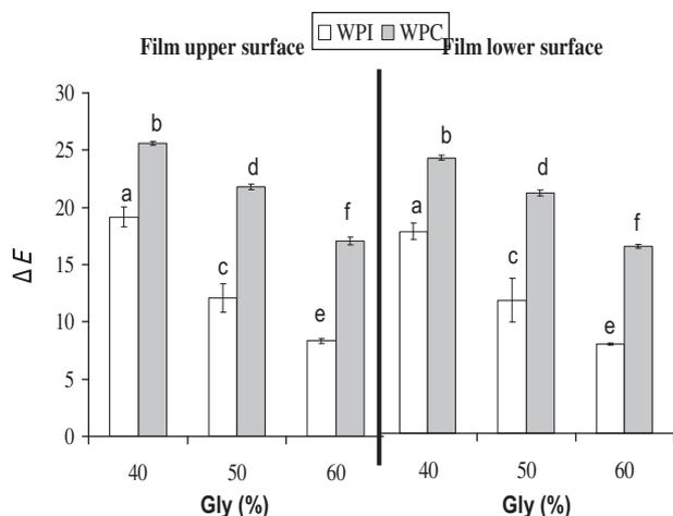
**Fig. 6.** Values (average  $\pm$  standard deviation,  $n = 4$ ) of  $\Delta E$  for the upper and lower surface of 10%(w/w) WPI- and WPC-edible films, with various glycerol (Gly) contents. Means labeled with the same letter do not statistically differ from each other ( $p > 0.05$ ).
