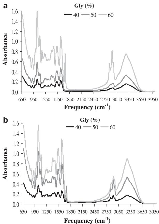
Fig. 3. FTIR absorbance spectra of 10%(w/w) WPI- (a) and WPC- (b) edible films, with various glycerol contents.
