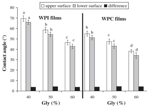
**Fig. 1.** Water contact angle values (average  $\pm$  standard deviation,  $n = 10$ ) for upper and lower surface of 10%(w/w) WPI- and WPC-edible films, with various glycerol (Gly) contents. Means labeled with the same letter do not statistically differ from each other ( $p > 0.05$ ).
