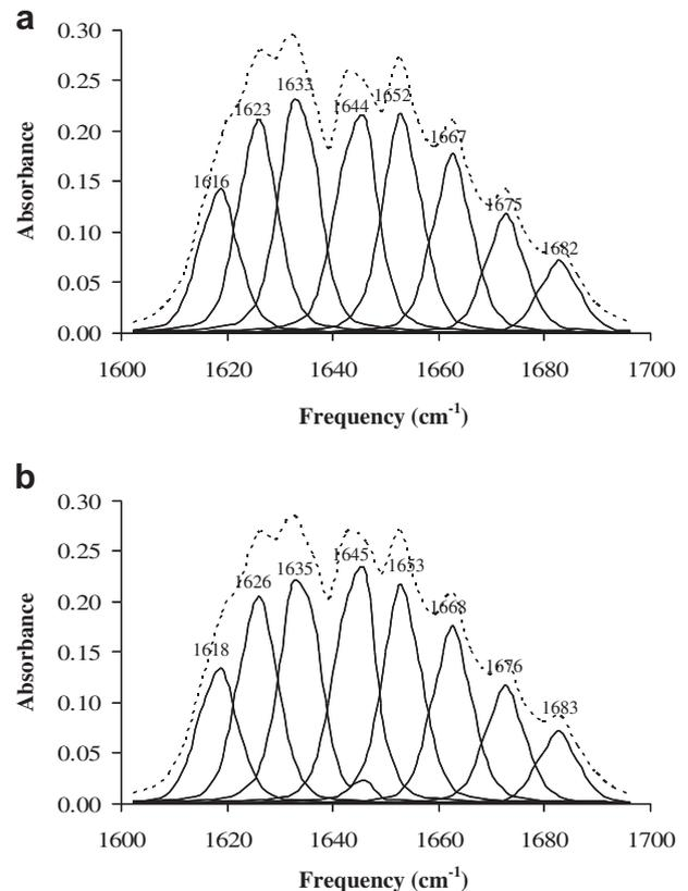
Fig. 4. Fourier self-deconvolution and curve-fitting of FTIR absorbance spectra, under attenuated total reflectance (ATR) mode, in the  $1600\text{--}1700\text{ cm}^{-1}$  region (amide I), of 10%(w/w) WPI- (a) and WPC- (b) edible films, with 50%(w/w) glycerol.
