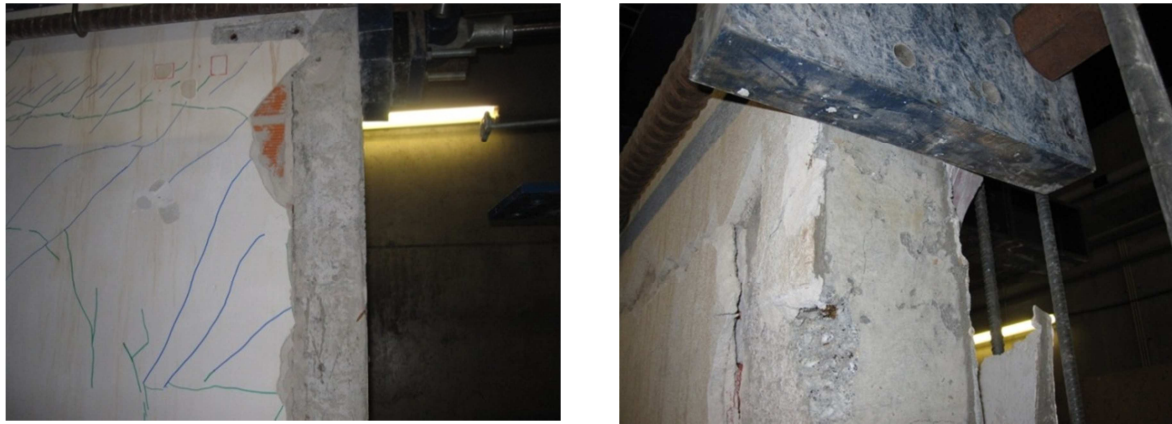
Figure 15: a) masonry/RC frame rupture; b) left column shearing failure
