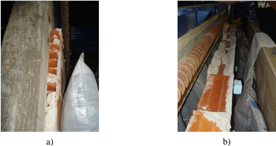
Figure 21: Out-of-plane expulsion: a) an intermediate phase of the test; b) complete separation of the masonry panel from the RC frame
