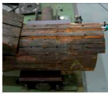
a) Shear failure beyond the step
