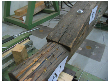
(b) Screws and internal bolt to strength the rafter-tie beam connections
