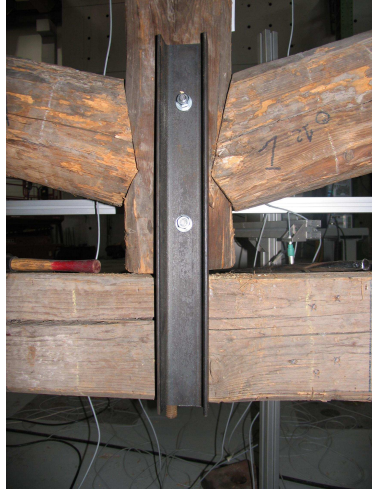
(a) UPN profile preventing the out-of-plane movements in the king post-tie beam connection
