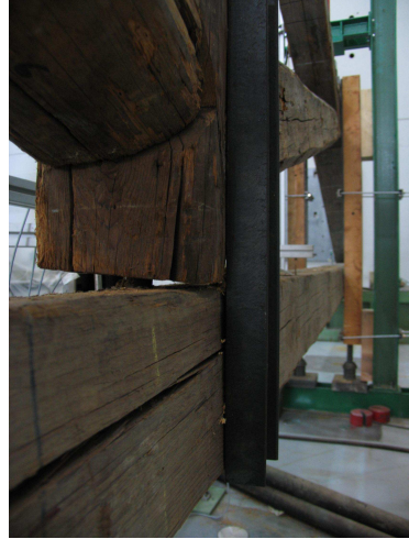
(a) UPN profile preventing the out-of-plane movements in the king post-tie beam connection
