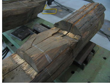
(b) Failure of the rear step
