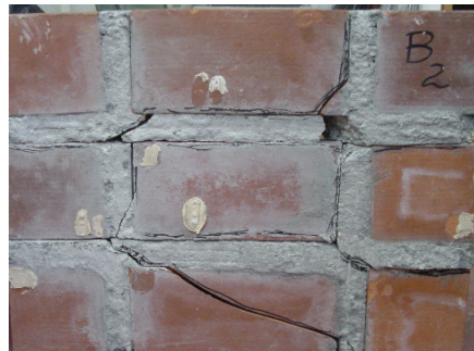
Figure 6 – Failure mode of the panels for series 1: (a) Panel 1; (b) Panel 2; (c) Panel 3.
