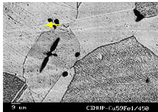
Fig. 6. Iron rich phase present at the microstructure of a studied alloy of the Cu–Zn–Fe system.
