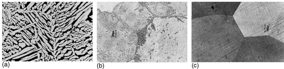
Fig. 5. Effect of aluminium additions in the microstructure of Cu–Zn base alloys.
