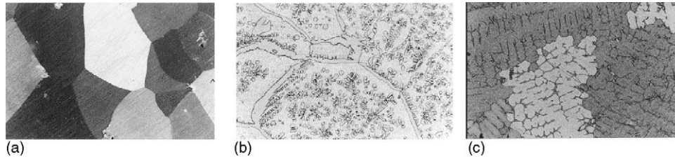
Fig. 2. Effect of tin additions in the microstructure of Cu–Zn base alloys.
