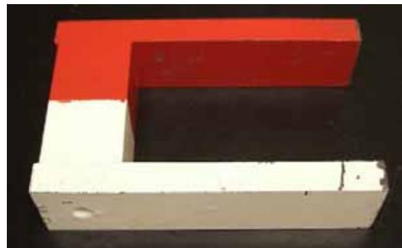
Figure 6. Permanent magnet used to induce a voltage in the coil.
