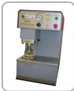
Aparelho – Digital bursting strenght tester
