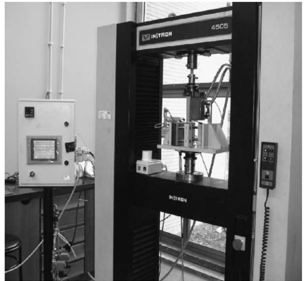
Fig. 4. View of the equipment installed in a universal testing machine.
