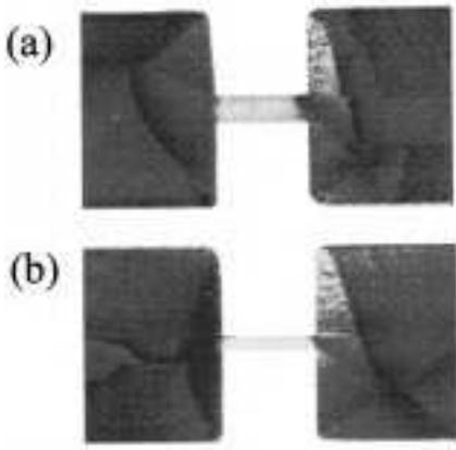
Fig. 4. MFM images of the bridge structure with (a)  $w = 1 \mu\text{m}$  and (b)  $w = 0.5 \mu\text{m}$  in the demagnetized state. The narrow regions with  $w = 0.5, 1 \mu\text{m}$  show a single domain state, while multidomains are seen in the wide wires.
