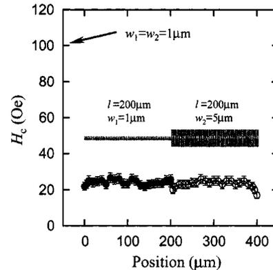
Fig. 1. The variation of the switching field as a function of position for the wire junction structure ( $w_1 = 1 \mu\text{m}$ ,  $w_2 = 5 \mu\text{m}$ ), measured every  $10 \mu\text{m}$  along the wire length. The arrow indicates  $H_c$  in the fixed width wire ( $w_1 = w_2 = 1 \mu\text{m}$ ) obtained by MR measurement.
