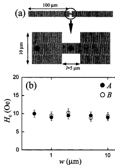
Fig. 3. (a) Schematics of the bridge structures, which have a narrow region with a length  $l = 5 \mu\text{m}$  and a width  $w = 0.5\text{--}10 \mu\text{m}$  introduced in the center of the wire. The dots on the schematics denote the fixed positions **A** ( $50 \mu\text{m}$  away from the end of a wide wire) and **B** (center of the narrow wire) of the laser beam spots. (b) The variation in the switching field ( $H_c$ ) against the wire width of the narrow region.
