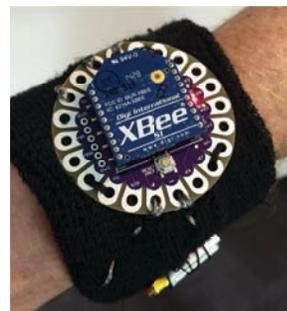
Figure 1. Wristband used to give haptic feedback.
