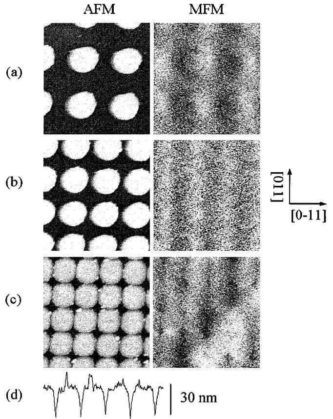
Fig. 3. AFM and MFM images of  $1 \mu\text{m}$  dot arrays of three different separations: (a)  $1 \mu\text{m}$ , (b)  $0.5 \mu\text{m}$ , and (c)  $0.1 \mu\text{m}$ , and (d) line scan across the  $0.1 \mu\text{m}$  dot array in (c) showing clearly that the dots are not connected.
