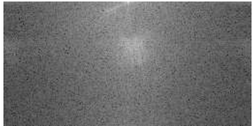
Figure 3: Power Spectrum of the image in figure 1. The range of circulus frequencies is represented by the width of the peak
