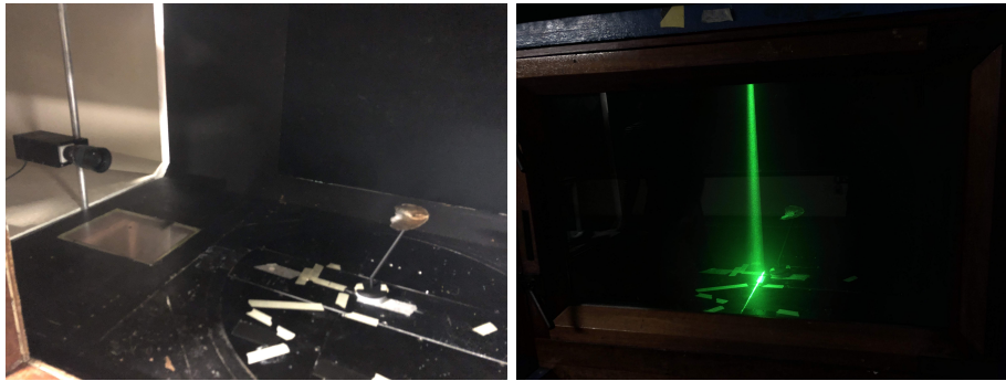
(a) Diaspore mounted on the support. (b) Green laser illuminating the wake.
