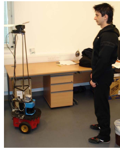
Fig. 3. Mobile robot with laser and camera.
