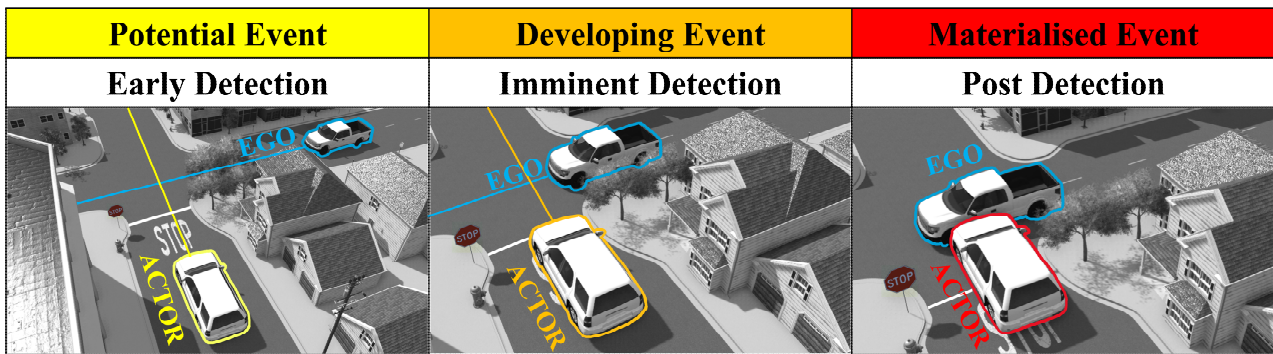
Fig. 1. Hazardous event lifecycle example of environmental occlusion that masks the presence of oncoming traffic and cause collision.
