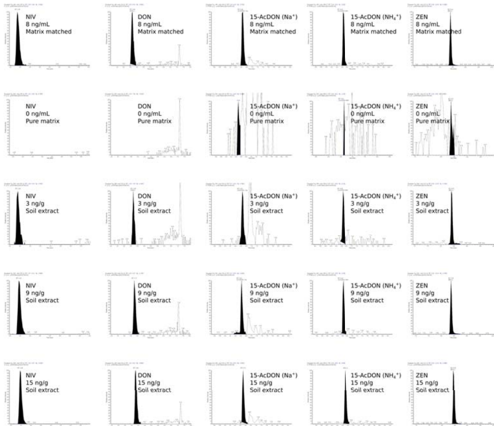
Figure A3. Example chromatograms of nivalenol (NIV), deoxynivalenol (DON), 15-acetyl deoxynivalenol (15-AcDON), and zearalenol (ZEN) measured in the matrix-matched calibration, pure matrix, and in soil extracts from RefeSol02A spiked at the levels 3, 9 and 15 ng g -1 soil.
