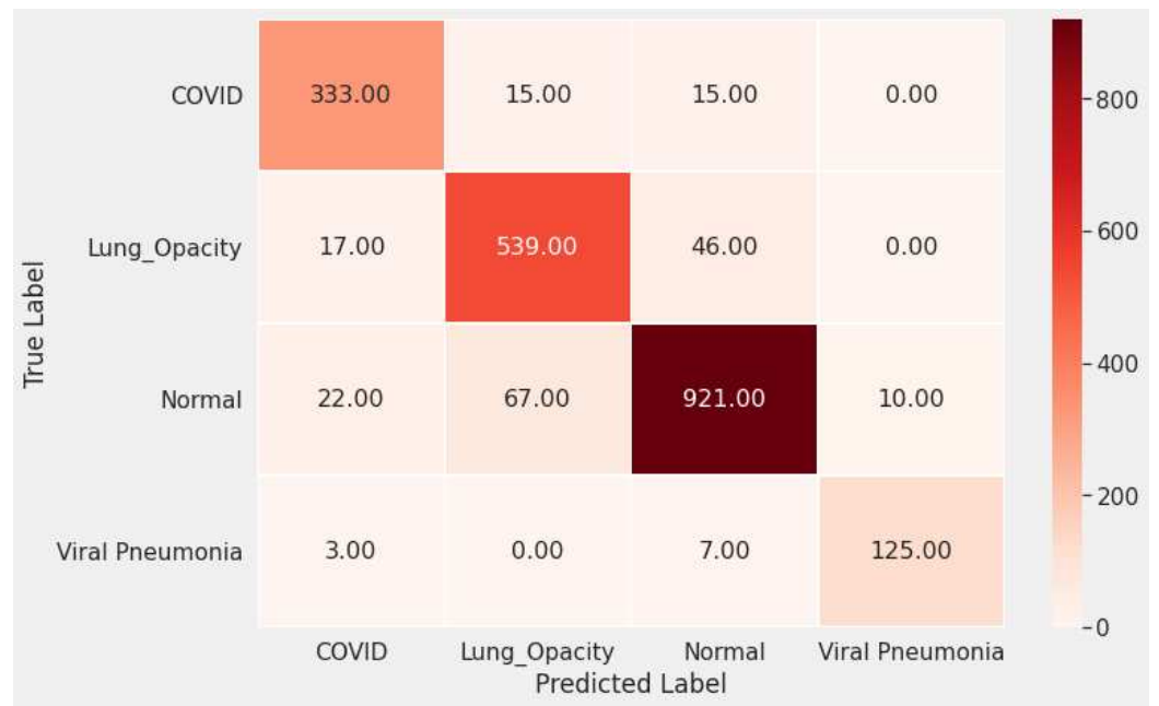
Figure 5. The confusion matrix of the standard MobileNetV2 shows many false negative and false positive classifications, especially for the COVID-19 cases.
