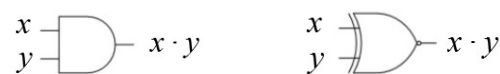
Figure 1. Basic implementation scheme of a SC multiplier in the (0..1) range (AND gate, left) and in the (-1..1) range (XNOR gate, right).
