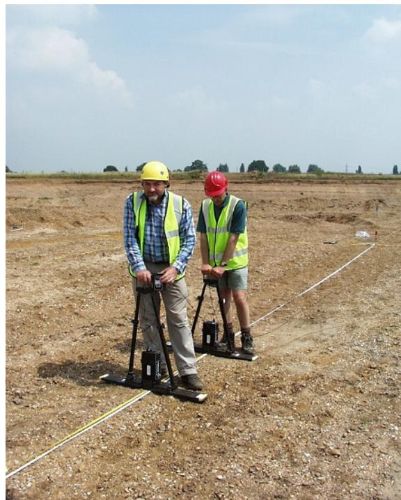
Figure 7. The Pulse Ekko 100 with 100 MHz antennae, in use on the ‘5m bench’ at Holme Pierrepont.
