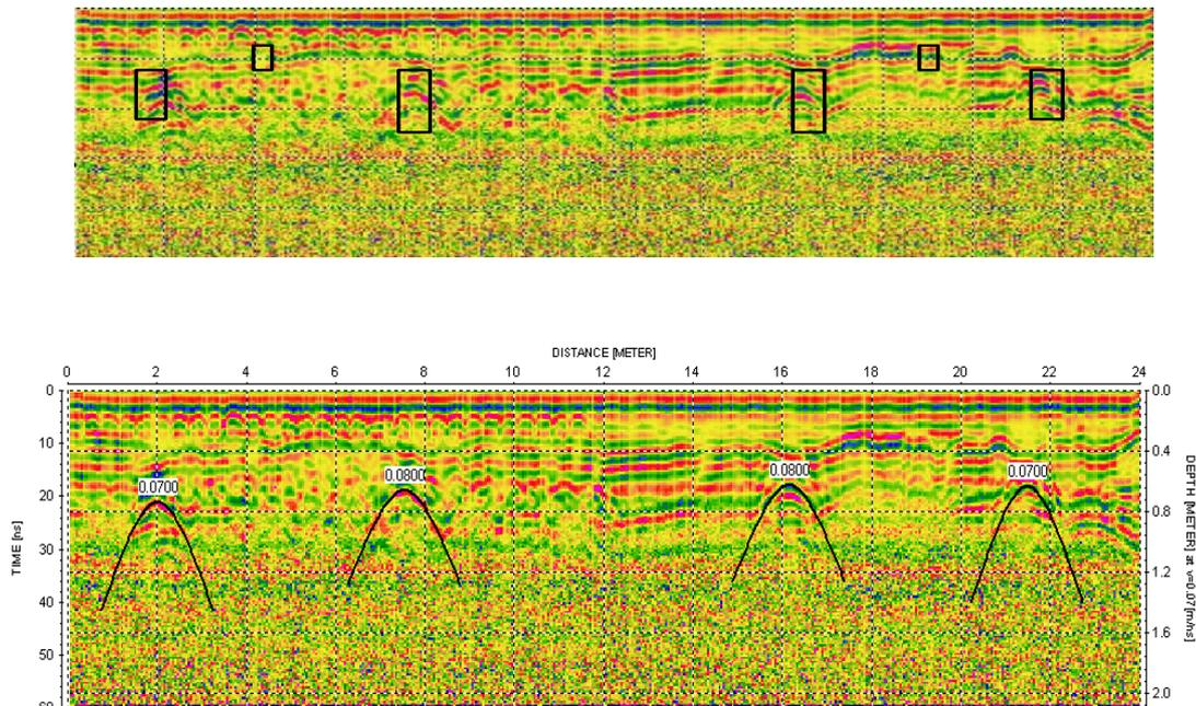
Figure 15. Radargram from the TRL road test track illustrating a number of features. The black squares in the upper image shows the location of voids. GPR hyperbolae from the voids are highlighted in the lower image where they have been used to estimate radar velocities.
