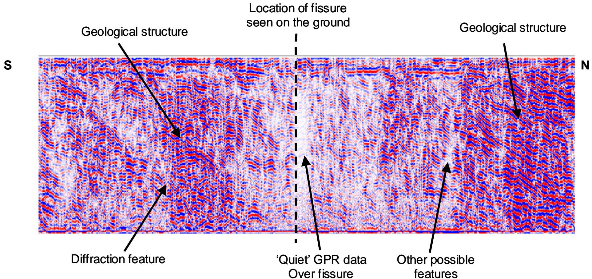
Figure 4. Summary of the general features seen at Houghton Hill farm. The fissure is shown as a shadow feature. Considerable geological structure is observed. Other shadow zones may suggest smaller scale fissures. A diffraction feature is also seen at depth and could also be a fissure. Assuming a radar velocity of  $0.0715 \text{ m ns}^{-1}$ , the section has a full depth extent of 7m.
