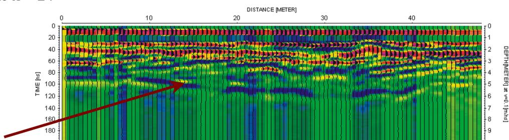
Figure 9. Radargrams of 50 MHz data from the ‘10 m bench’ at Holme Pierrepont. Data were collected along five lines in the x direction. Depth conversion based on a velocity of  $0.1 \text{ m ns}^{-1}$ . The Mercia Mudstone reflector is indicated by an arrow.
