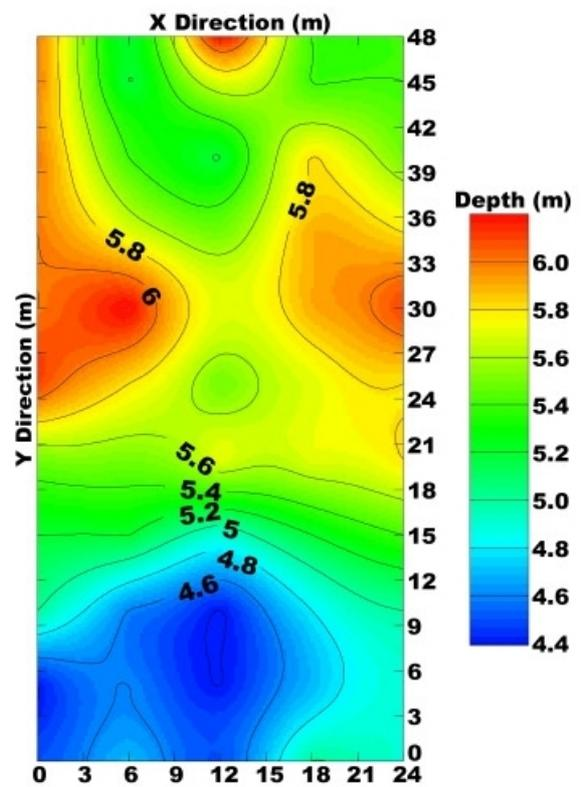
b) '5 m bench', depth to base of aggregate
