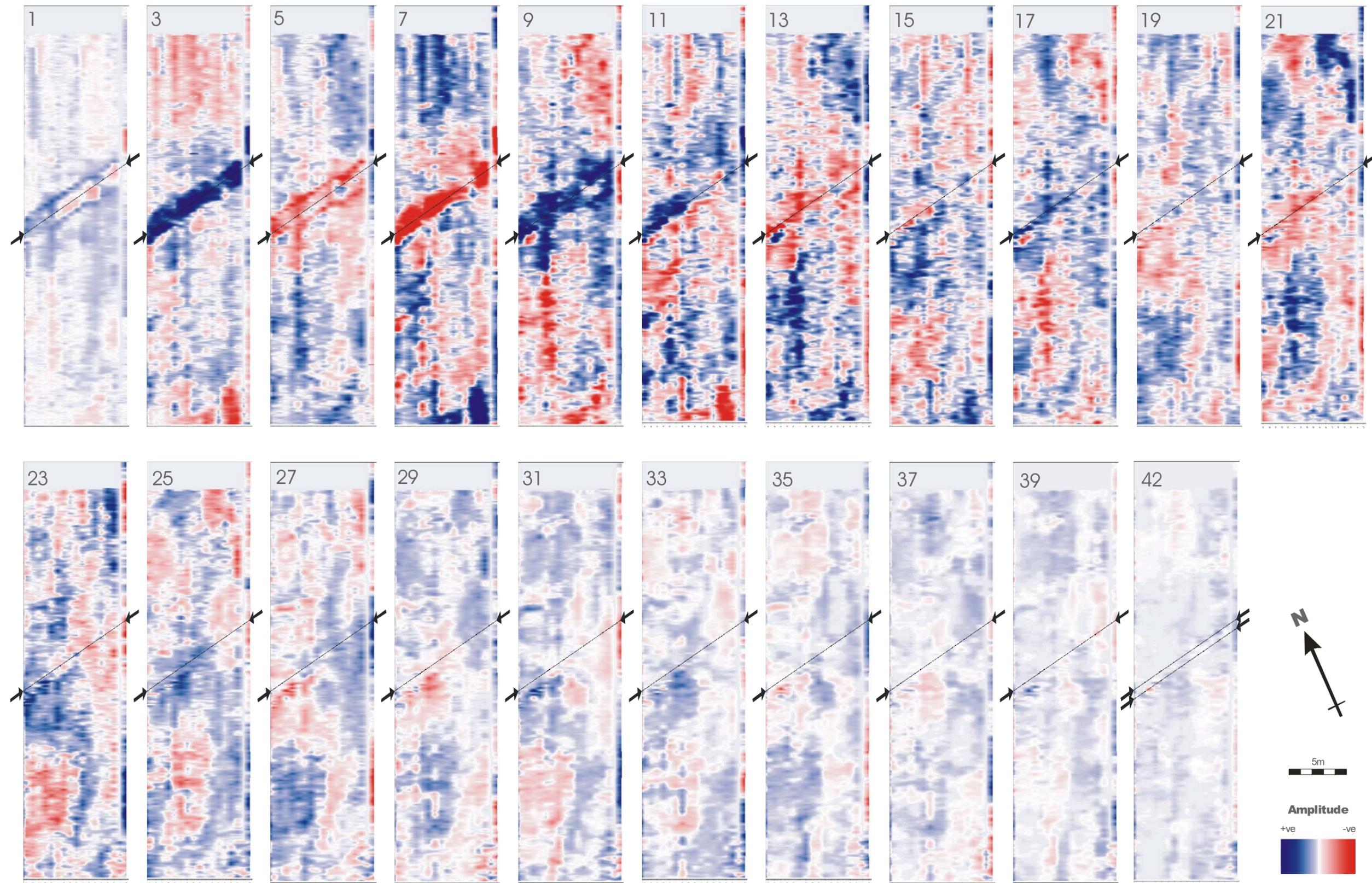
Figure 3. Time slices of GPR generated from a 3D data representation. Each successive map represents increasing depth. The location of the known fissure is highlighted. Depth slices from 1 to 42 represent the surface level down to a depth of approximately 1m, assuming a radar velocity of  $0.0679 \text{ m ns}^{-1}$ .
