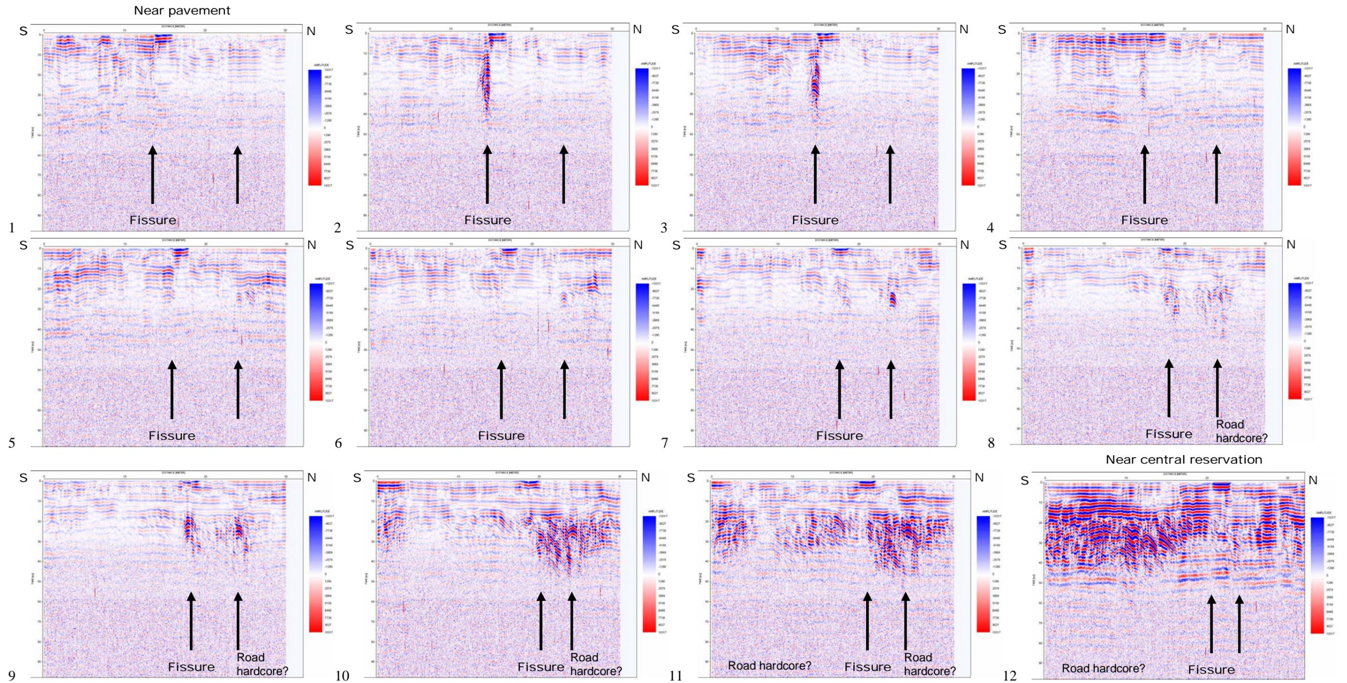
Figure 2. Radargrams of 250 MHz data for 12 of the lines conducted along the northbound carriageway of the A690. As highlighted, the fissure can be seen on almost all of the cross-sections. Assuming a radar velocity of  $0.0679 \text{ m ns}^{-1}$ , each section has a full depth extent of 6.65 m, with useful penetration not exceeding 3 m.
