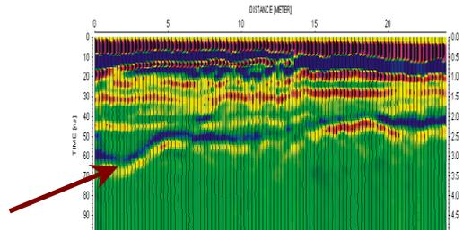
Figure 8. Radargrams of 100 MHz data from the '5 m bench' at Holme Pierrepont. Data were collected along five lines in the x direction and one line in the y direction. Depth conversion based on a velocity of  $0.1 \text{ m ns}^{-1}$ . Mercia Mudstone reflector indicated by an arrow.
