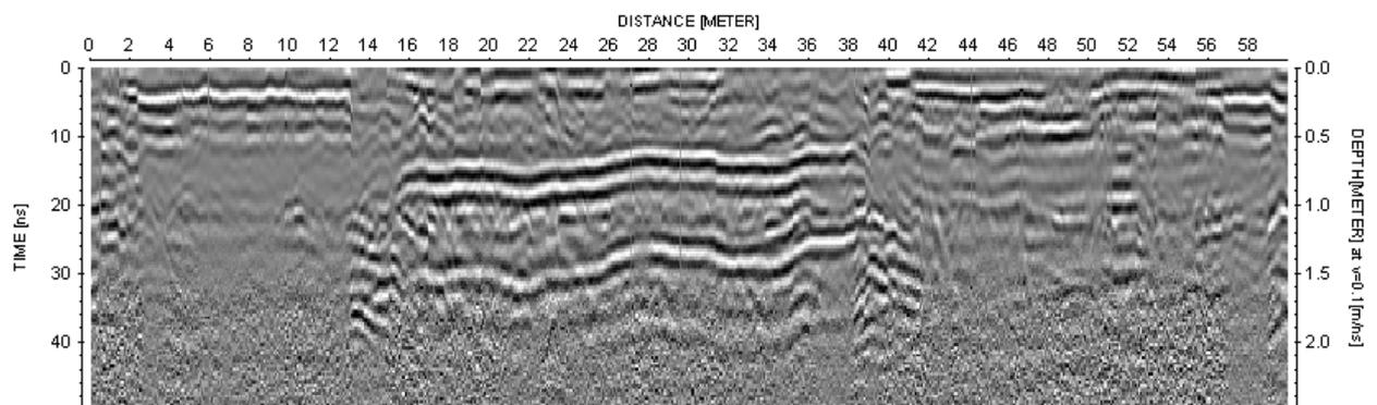
Figure 16. Radargram from Calverton Colliery, Nottinghamshire. The strong sub-horizontal reflector between 15 and 38 m is from the concrete cap over the mine shaft.
