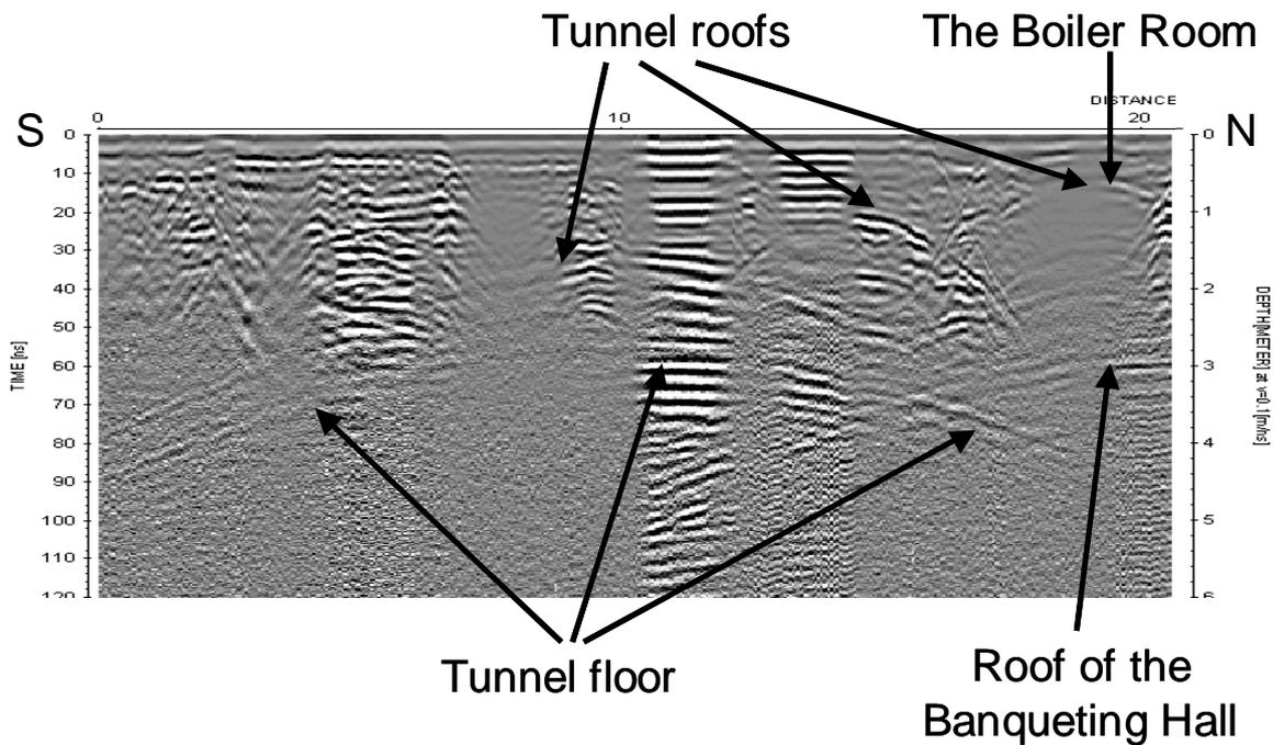
Figure 14. GPR results from over known tunnels. This traverse is taken from within Williamson’s house area. This image shows the roof and floor of the “Boiler Room” tunnel, the roof of the “Banqueting Hall” and the roof and floor of one other tunnel.
