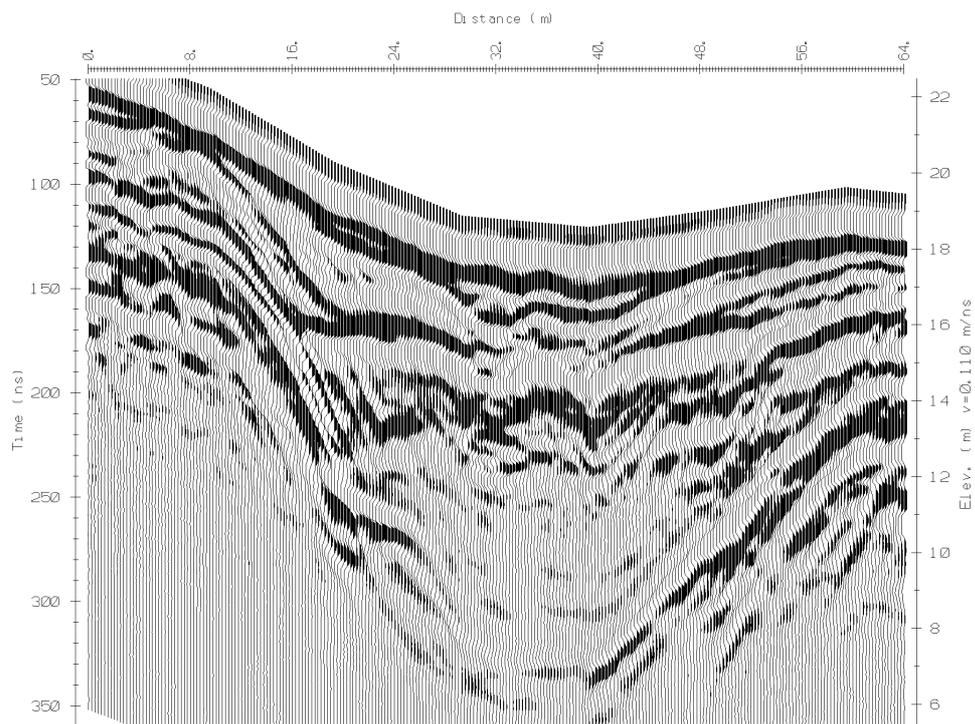
Figure 1. Example of a wiggle trace radargram. The reflections are interpreted as a kettle hole infilled with flat-lying overlapping sediments (after Busby and Merritt, 1999).
