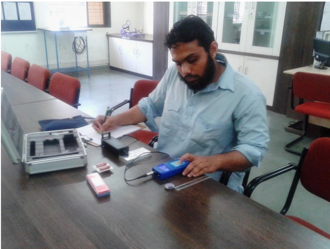
Figure 4.1 Measurement of Ra Values on Surface Roughness tester
