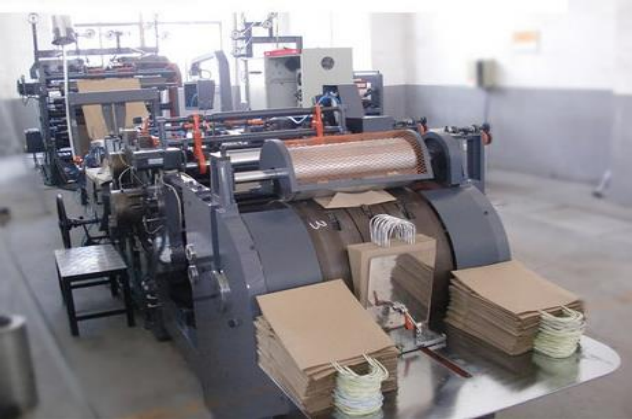
Fig 2.5 Automatic Paper bag making machine
