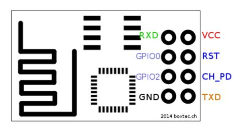
Above is a pin out diagram for the ESP8266 Module
