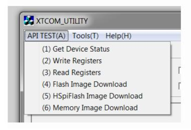
7. Select the .bin file to flash, and configure the correct destination address as in the readme.txt file (*For Example: boot\_v1.1.bin @ 0x00000*)
