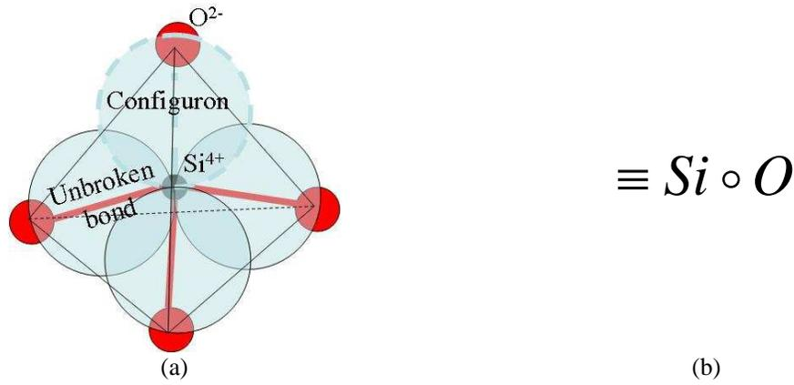
**Figure 1.** Configurational unit of amorphous silica (tetrahedron [SiO<sub>4</sub>]), its bond model and designation. (a) Bond model shown with three unbroken bonds and one configuron. (b) Bond model designation.
