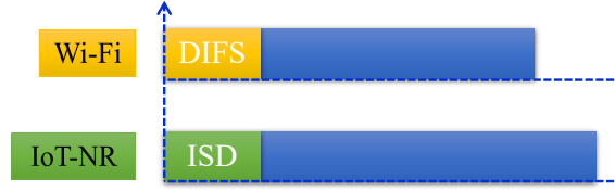
Figure 4.2: Initial contention for transmission between Wi-Fi and IoT-NR device over the unlicensed channel.
