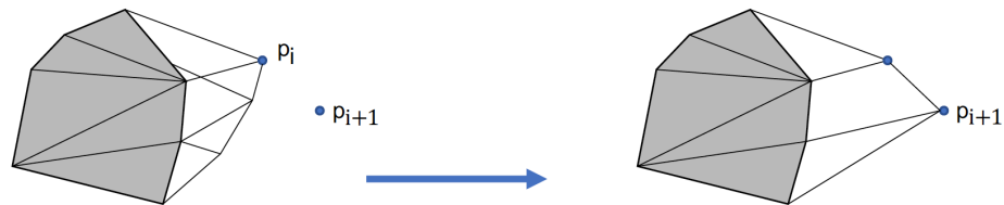
Figure 16 Quickhull algorithm adds the farthest point in the outside set to the convex-hull at each iteration. The outside sets, the facets, ridges, and vertices will be updated in each step. This process continues until there is no outside point.
