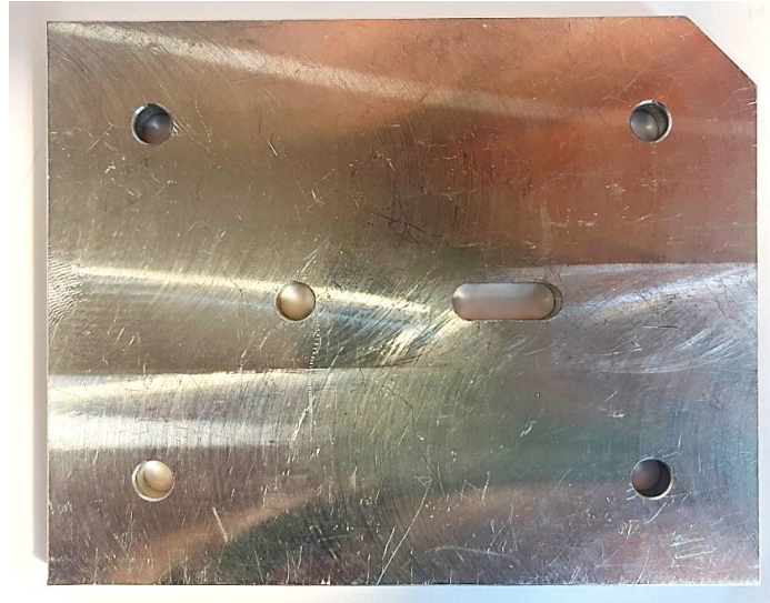
Figure 57. Machined Part B with hole and slot and four corner holes
