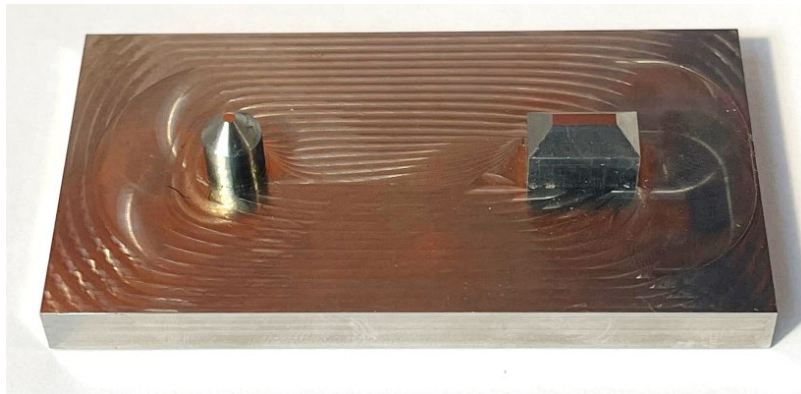
Figure 59. Machined functional gauge used for position of hole and slot inspection method
