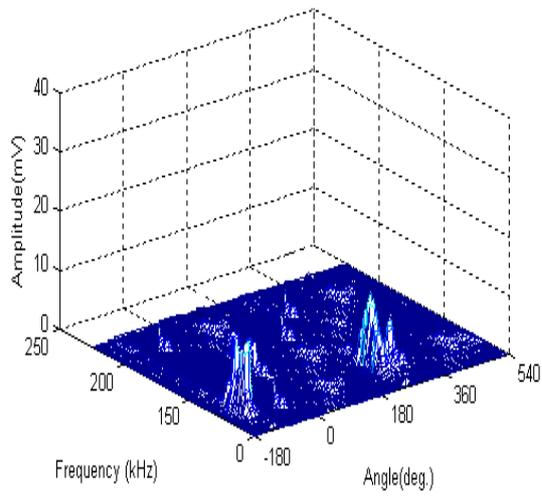
**Figure 7a:** Angular-frequency representation of the blocked injector
