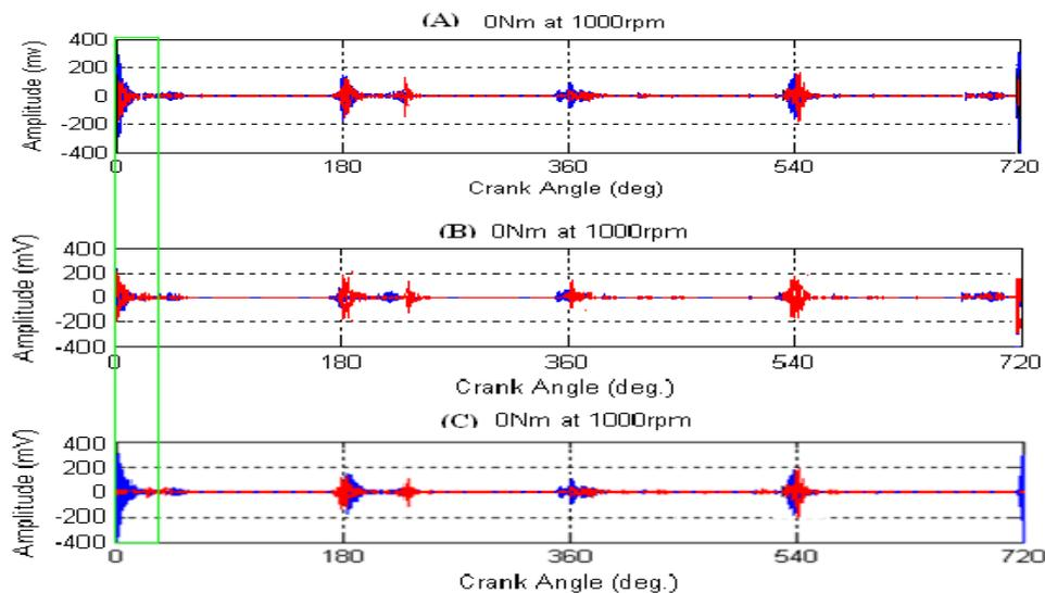
**Figure 2 AE signals in the angular domain.**
