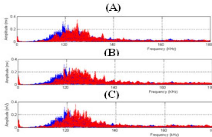
**Figure 3** Frequency spectra of the AE signals
