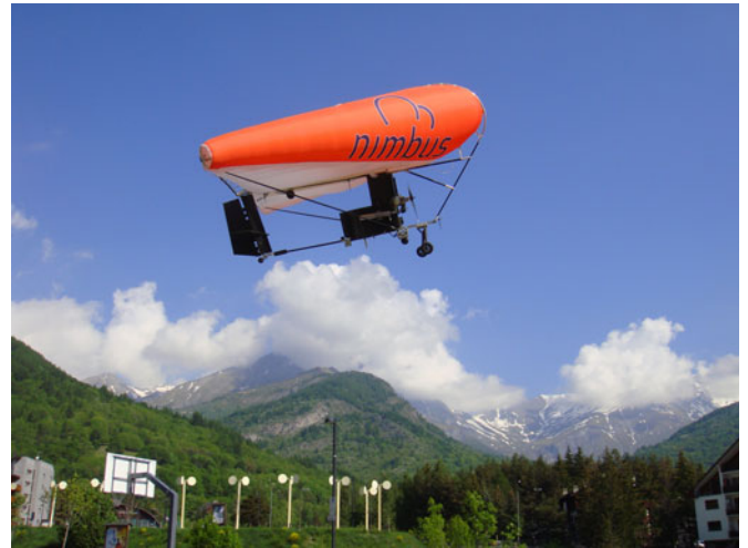
Fig. 4. Nimbus EosXi UAV platform.
