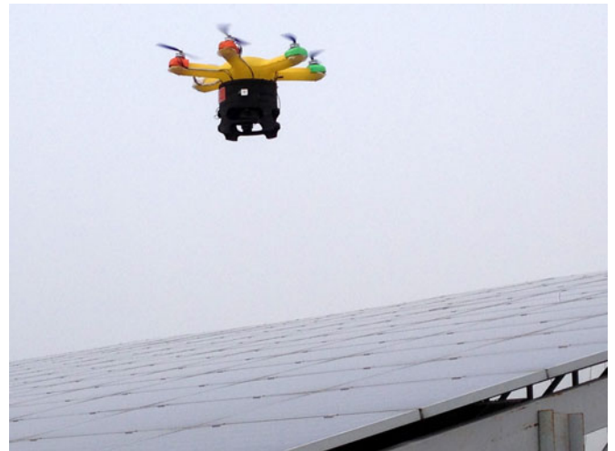
Fig. 5. Nimbus PLP6 during PV monitoring operation.
