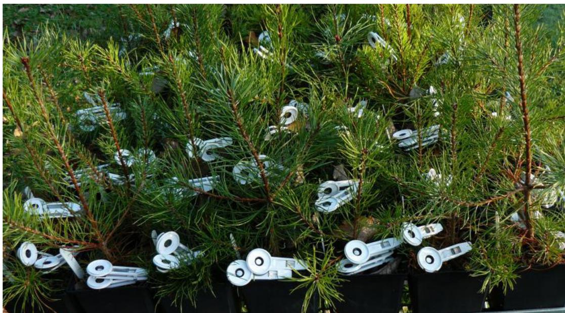
**Outdoor seedlings fitted with clips for dark acclimation prior to measurement of chlorophyll fluorescence.**
