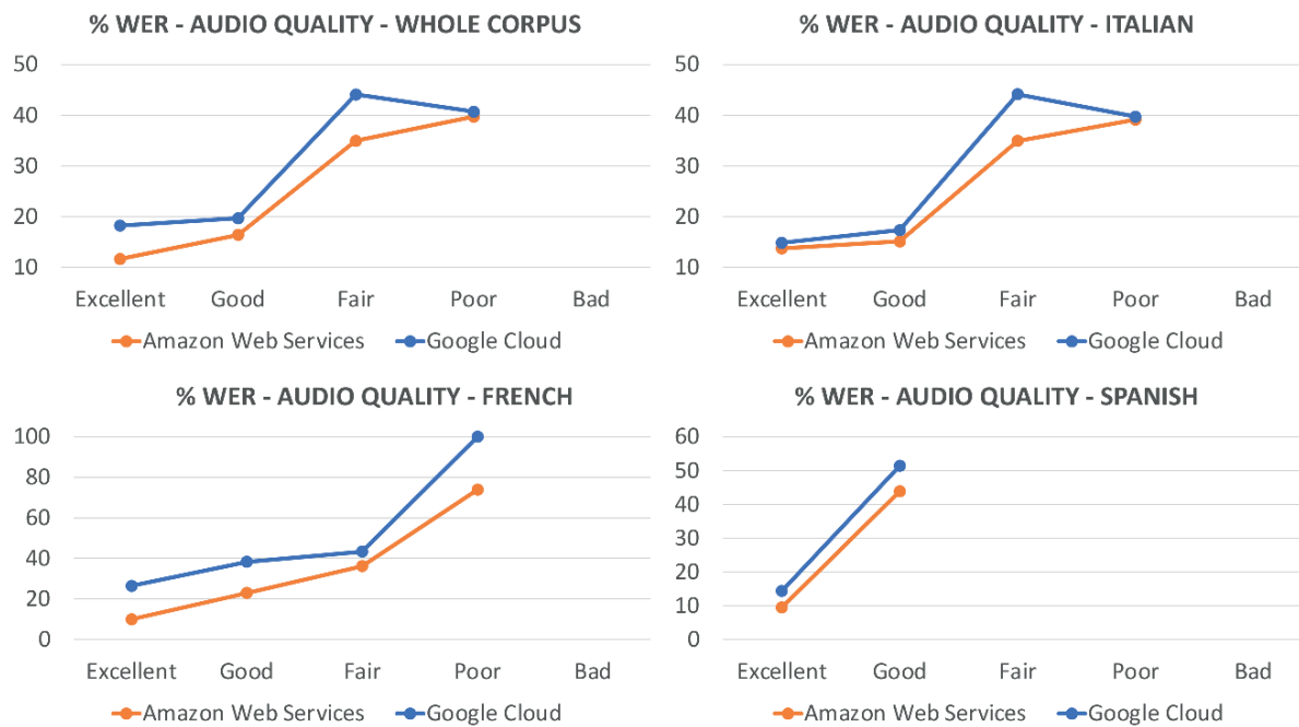
Figure 2: WER of GCS and AT with different audio quality - whole corpus and sub-corpora.
