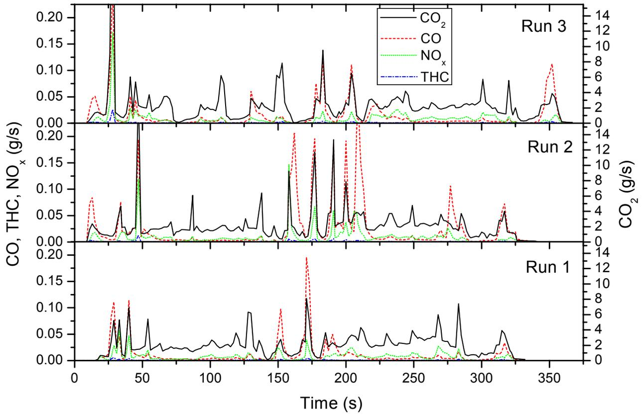
Figure 2: Emissions comparison for the three smooth runs
