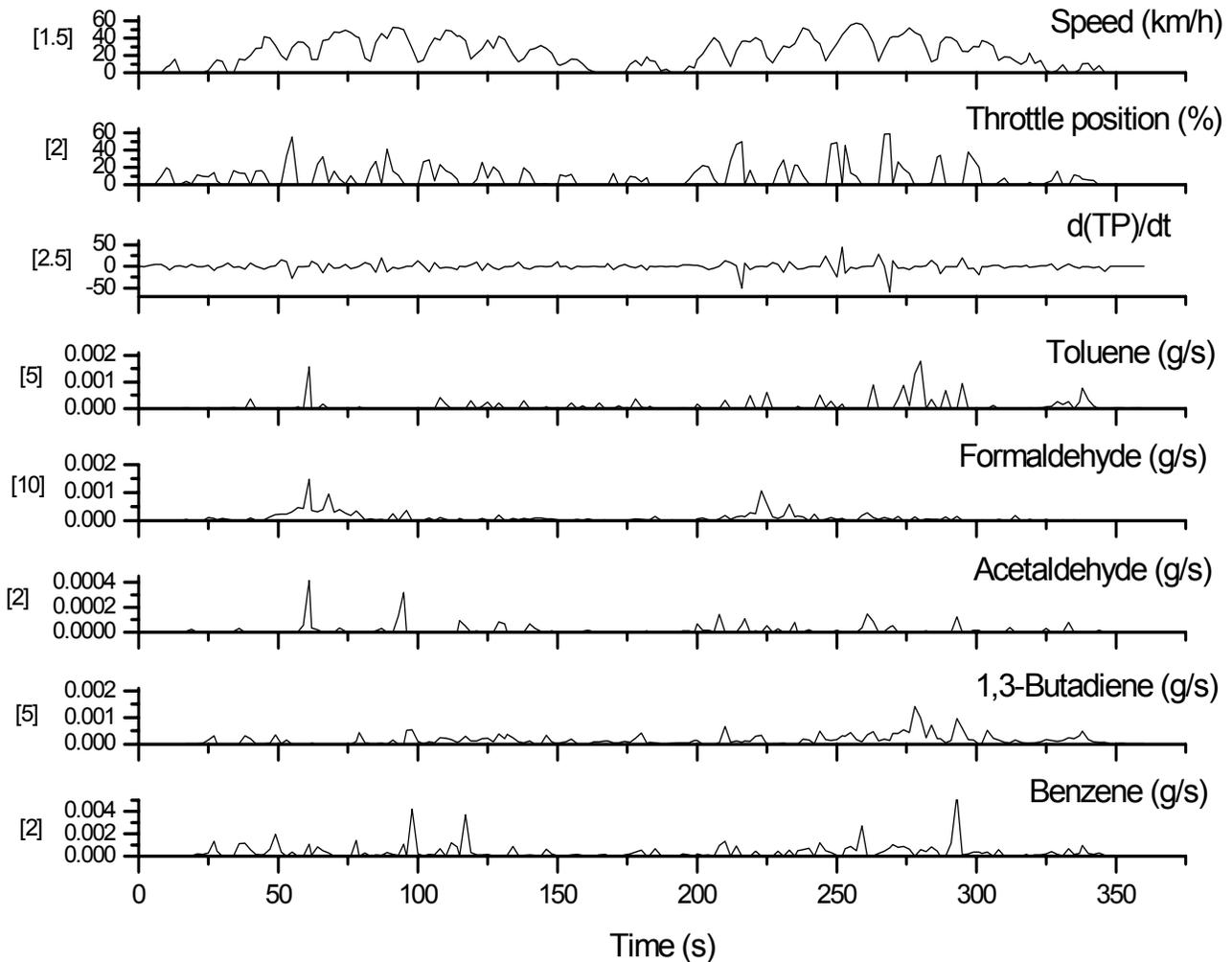
Figure 10: Non-regulated hydrocarbons from speed bump run 1 (numbers in square brackets to the left of y-axis are the ratio of 'speed bump' axis scale to 'smooth run' axis scale)
