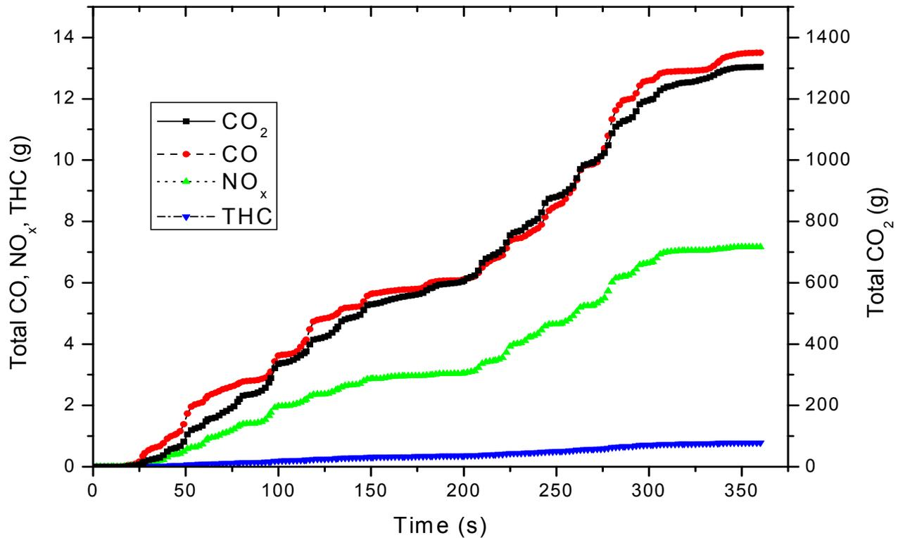
Figure 8: Cumulative emissions plot of speed bump run 1
