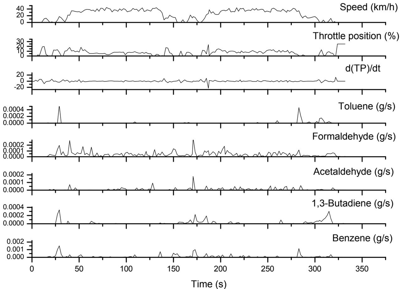
Figure 9: Non-regulated hydrocarbons from smooth run
