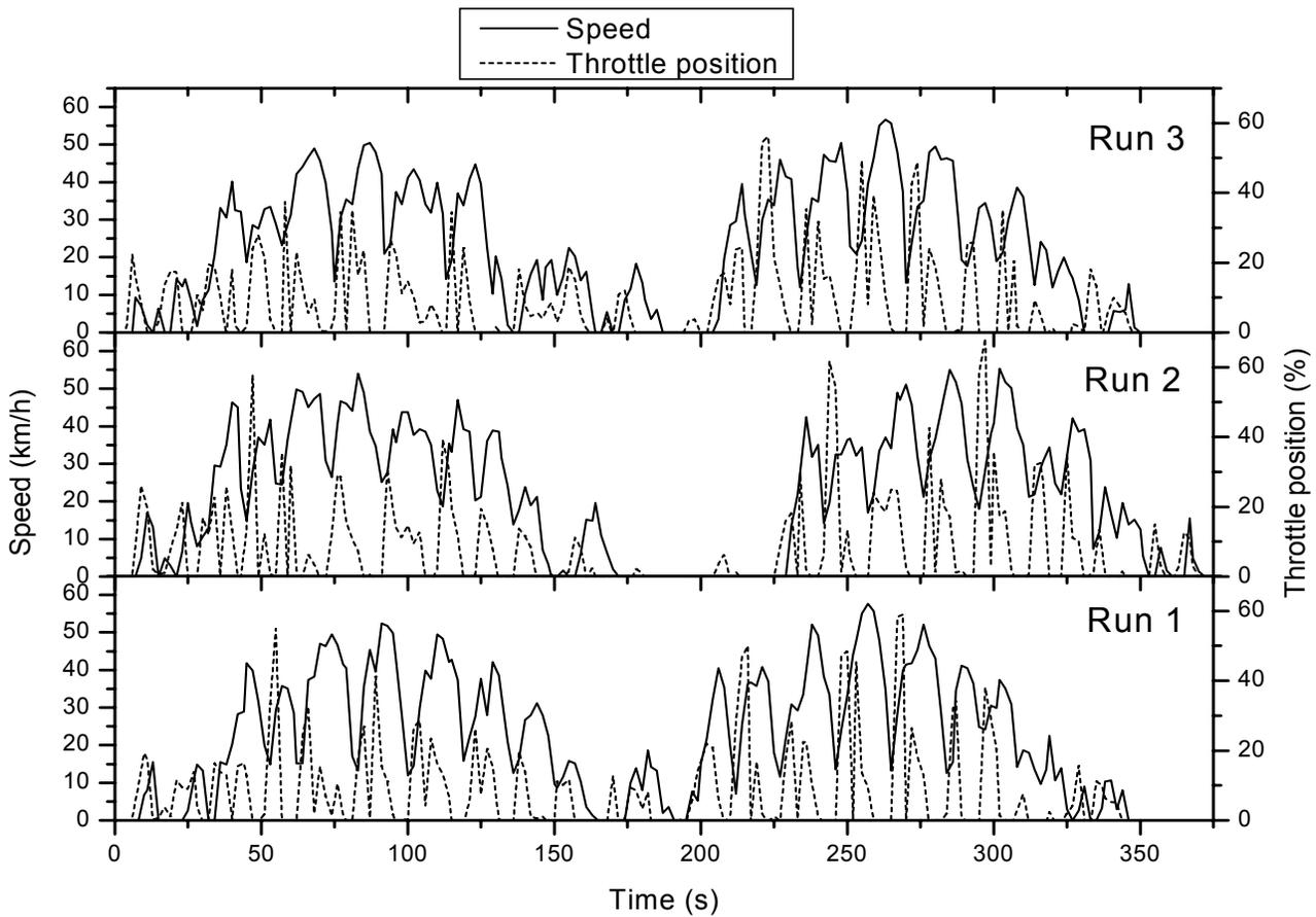
**Figure 5: Speed and throttle position for the three speed bump runs**
