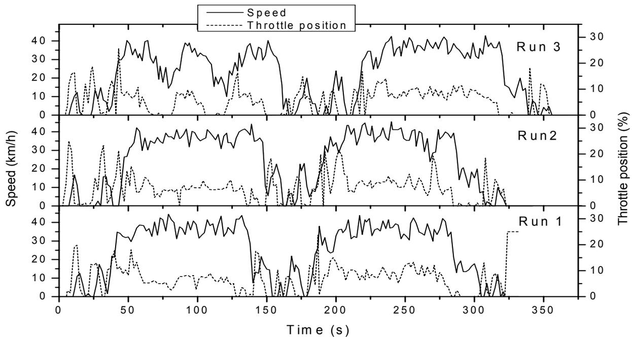
**Figure 1: Speed and throttle position for the three smooth runs**
