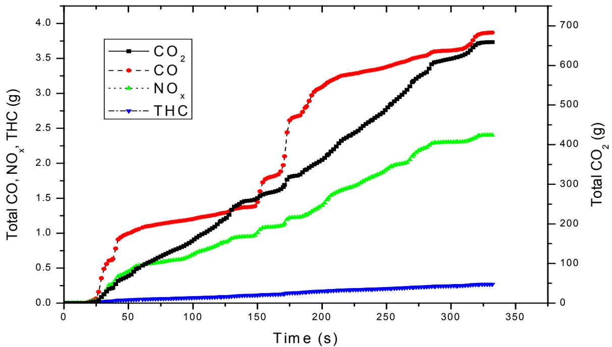
Figure 3: Cumulative emissions plot of smooth run 1
