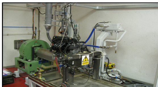
Fig. 1.1. Photograph of the study state engine rig.
