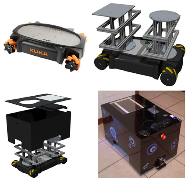
Fig. 2 Design process of KuBo. The overall height of the robot is about 30 cm and a new cover, made of black opal methacrylate, is mounted to an internal frame. The last picture shows the final prototype
