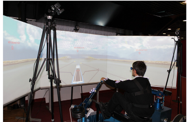
Fig. 1. The SPRINT rowing training system presented in an immersive configuration with three stereographic screens and motion capture.
