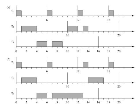
Figure 4. Under EDF, the number of preemptions may decrease when execution times increase: in case (a), where  $C_3$  is small,  $\tau_2$  is preempted by  $\tau_1$ , but this does not occur in case (b), where  $\tau_3$  has a higher execution time.
