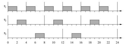
Figure 5. The condition in which all periods are multiple of the shortest period is not sufficient to guarantee a schedulability bound equal to one.
