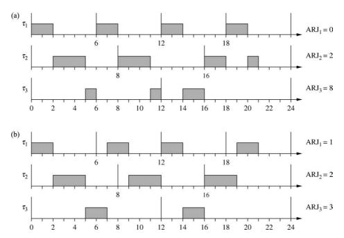
Figure 10. Response time jitter introduced under RM (a) and under EDF (b).
