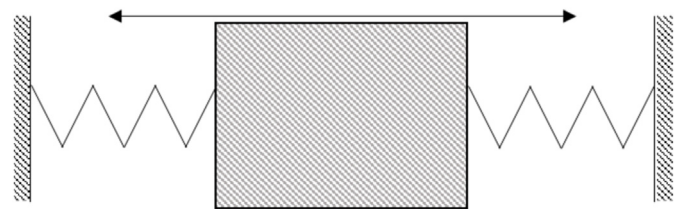
Fig. 9. A single degree of freedom mass between two springs used as an analogy for a parallel jointed rock mass.
