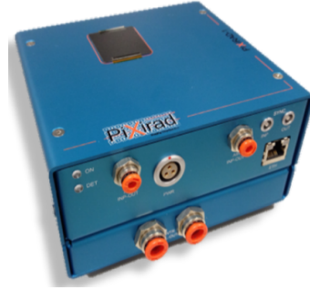
Figure 1: Pixirad-1 detector module unit
