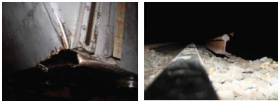
Fig. 4. The gas oil tank of the locomotive which was ripped on open line, and the long rail causing the accident [9]
